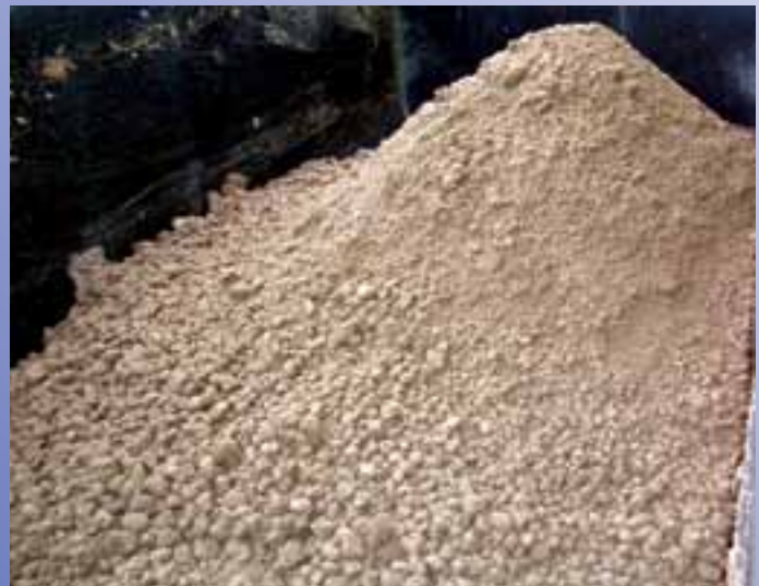
Dry granular discharge solids from the Screw Press
