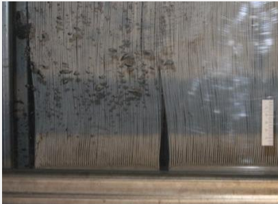
Coarse bubble air scour Source: GE Water (2011)
