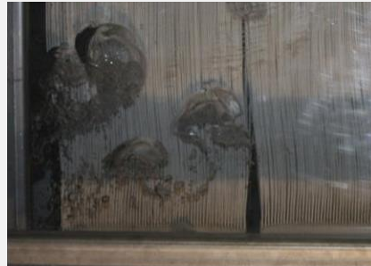
Gas sparging air scour Source: GE Water (2011)
