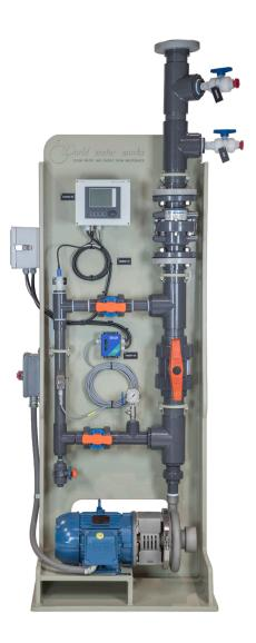
The stream is then discharged back into the tank, and water is recirculated until the pH reaches an acceptable range. The Ideal pH System recirculation pump is operated in with a Hand/Off/Auto switch. In hand, the pump will operate until it is turned off. In Auto, the pump will start and stop based on the control signal that determines if pH adjustment is needed at that time. The feed pump is controlled either locally on the pump, or from a 4/20 mA signal.
