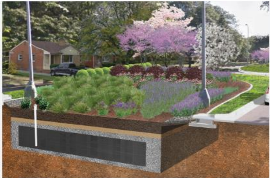
Rendering of New Landscaping Design and Underground Stormwater Storage Area (section view; approximately three years after planting)
