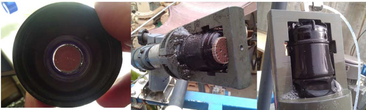
Figure 16 Left: DO Sensor lens scratching by media; Middle: Media trapped between probe and probe guard; Right: Probe/Probe guard retrofitted with an air scouring device.
