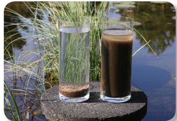
SVI5 comparison of aerobic granular sludge (left) and conventional activated sludge (right)
